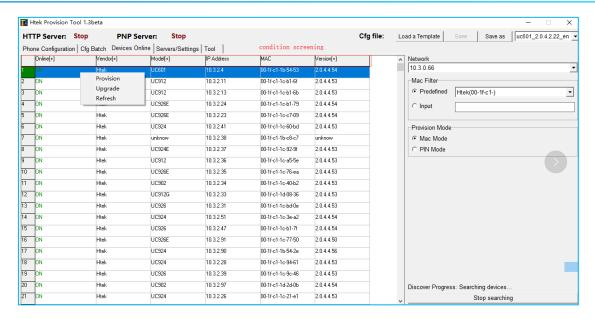
The results of the search are presented as shown in the table above. The head can be used for the screening of device model and version number.
